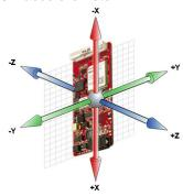
The module contains a 3D accelerometer (up to 16g), which can be used for a variety of custom specific (M2M) applications. Accelerometers are useful for measuring movement, speed, g-forces and vibration of the object. The accelerometer and advanced embedded firmware enables a very low-power battery solution.
